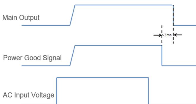
Figure 5. Power Good Time Sequence
